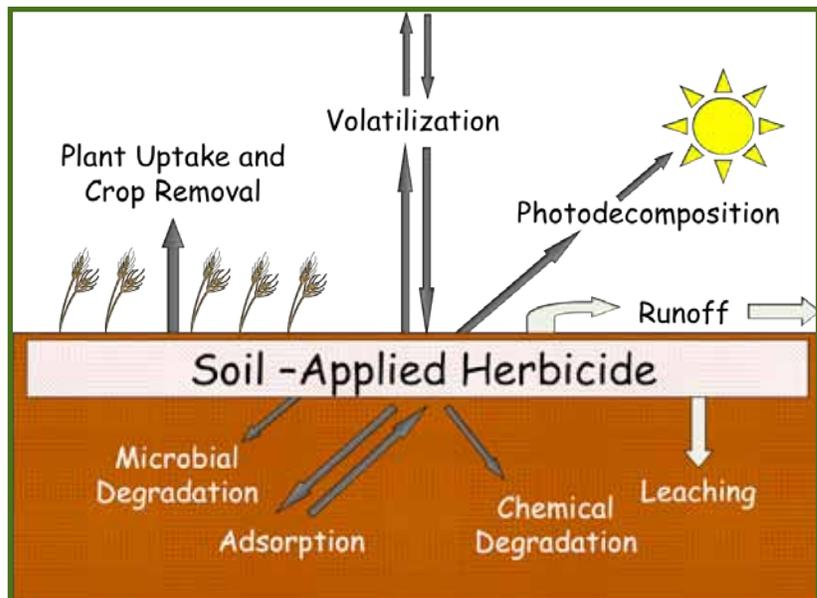
**Figure 5.** Factors affecting the fate of soil-applied herbicides.
